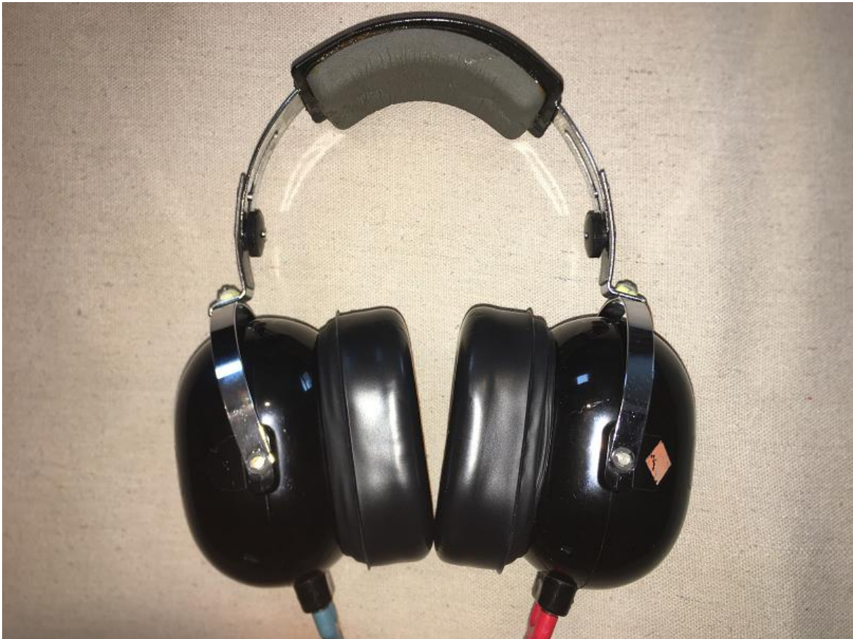
Maico “Auraldomes” Headset with TDH-39 Elements and Kore Aviation Plush Silicone Gel Cushions
