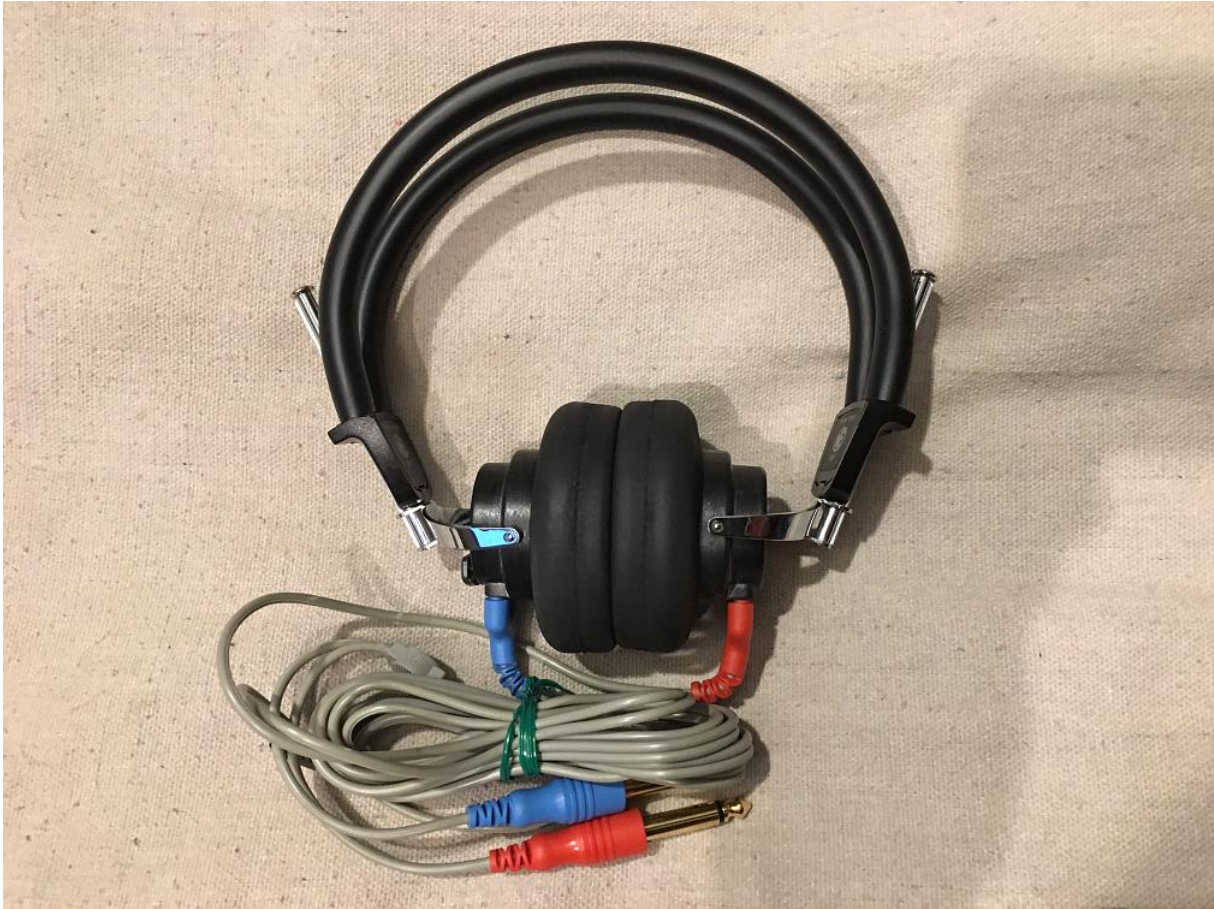
Madsen Headset with TDH-39P (296D000-1) Elements and Wilfan Electronics MX-41/AR Cushions
