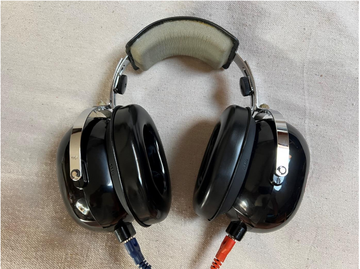
Aural Research AR-100 “Auraldomes” Headset with TDH-49P Elements and David Clark 40863G-02 Gel Cushions
