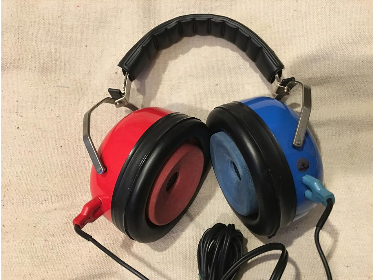
Amplivox Audiocups Headset with Pierce-Roberts Red and Blue MX-41/AR Cushions and TDH-39P (296D000-1) Elements
