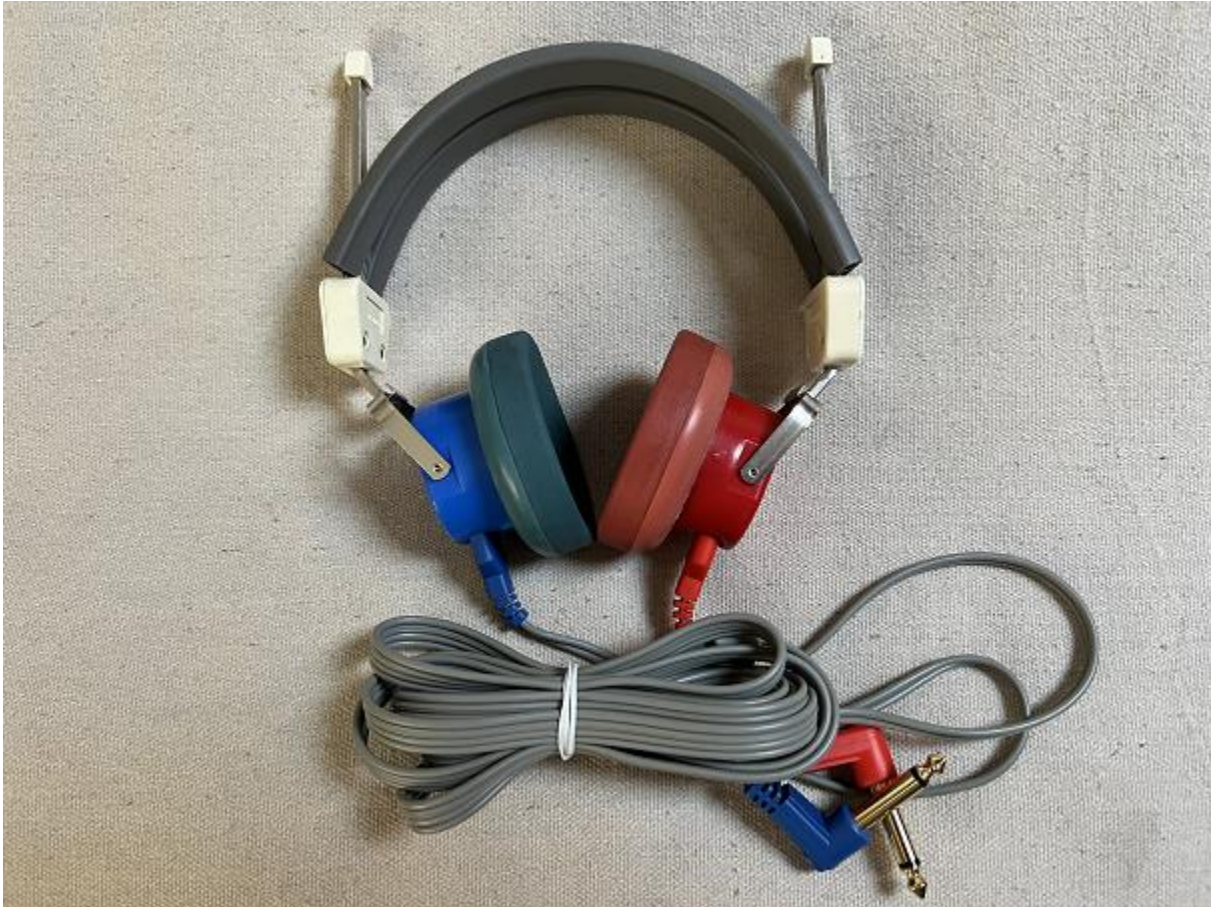
Qualitone Headset with Pierce-Roberts Red and Blue MX-41/AR Cushions and TDH-39P (296D000-1) Elements
